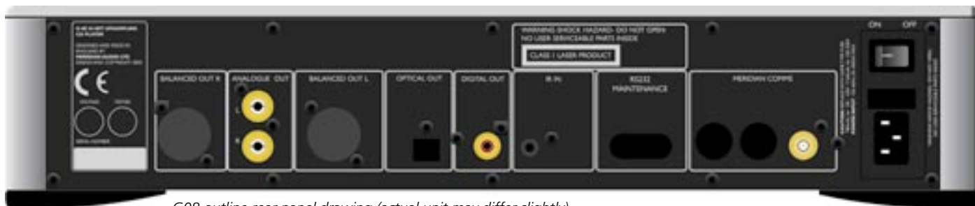
G08 outline rear panel drawing (actual unit may differ slightly)
