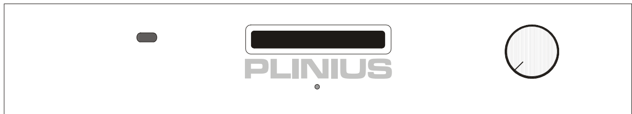
Front Panel Layout Showing Volume Knob, Vacuum Fluorescent Display, And Display LED
