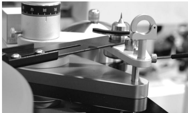
FIG. #1: THE PROPER WAY TO USE THE ALIGNMENT JIG. THE PICTURE SHOWS A 12.6 BEARING, THE ADJUSTMENT IS THE SAME.
