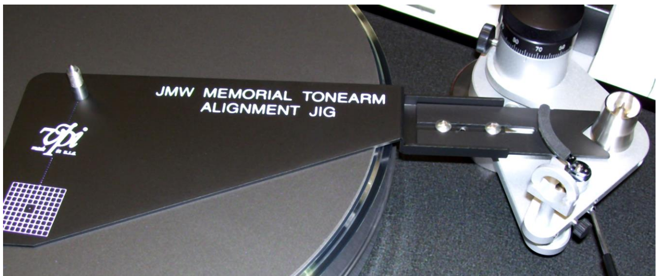
FIG. #1: THE PROPER WAY TO USE THE ALIGNMENT JIG.
